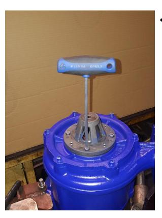
Remove the fixing screws 4x M6x16 DIN 6912
